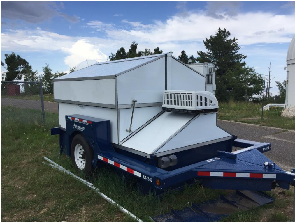
Figure 4. The Dog House in its closed position prior to lowering the trailer bed into the operational position at the Mt. Lemmon site near Tucson AZ.
