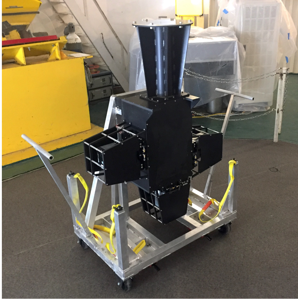
Figure 4: The complete Chimera instrument loaded on the transport cart
